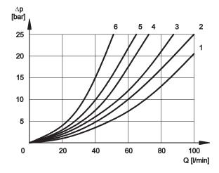
For pressure drops between A and B lines of spools S10, S20, S21, S22 and S23, which are used in the regenerative diagram, refer to curve 5.
