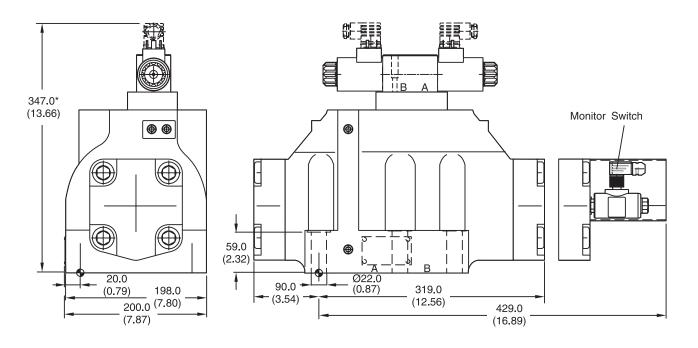
\* Please add for each sandwich plate +40mm (1.58") (pressure reducing valve, pilot choke meter-in/-out).
