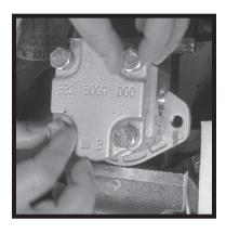
16) Install hardware (bolts and washers). Thread the fasteners into the mounting flange and tighten alternately or cross corner. Torque diagonally opposed fasteners to correct torque. Do not lubricate fastener threads before assembly.
