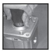
**3)** Press seal to a depth that is just deep enough to allow installation of the snap ring.
