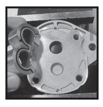
8) Assemble the front thrust block into the mounting flange, sealing parts can be fixed with grease. Orientation is rotation sensitive for pumps!
