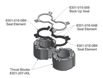
The proper seal installation is very important. If these seals are assembled upside down they will most likely fail in a short period of time under system pressure.
