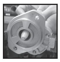
**10)** Insert shaft fully through mounting flange and remove sleeve.
