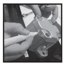
1) Place the unit in a vise with the drive shaft pointling down. Caution: DO NOT GRIP ON OR NEAR ANY MACHINED SURFACES DURING ASSEMBLY OR DISASSEMBLY. Match-mark all sections. Be sure to align these marks when reassembling.
