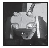
2) Use a metric wrench to remove the 4 cap screws.
