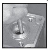
1) Clean seal bore thoroughly. When installing metal OD seals apply adhesive to the seal OD and the bore ID. Rubber OD seals do not require adhesive, instead a lubricant should be used on the OD.
