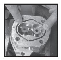
**13)** Install section seal. Use grease to hold into groove.
