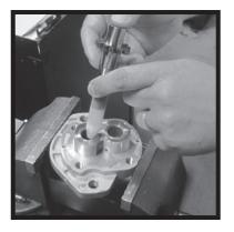
9) Slide the mylar shaft seal sleeve over the drive shaft. Lubricate the sleeve with grease to lubricate the shaft seal during assembly.
