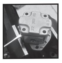
3) Lift off the port end cover. If prying is necessary, be careful not to damage the machined surfaces
