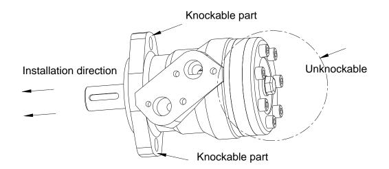
The motor cannot be installed with force or in distortion. Do not take away the plastic stuff before the pipe circle and the oil pipe are installed.
