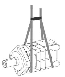
The motor cannot be installed with force or in distortion. Do not take away the plastic stuff before the pipe circle and the oil pipe are installed.
