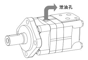
If the motor appears unsteady during low-speed operation, adding the backpressure, which is no less than 0.2 Mpa, can solve it.
