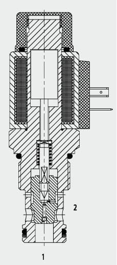
In the de-energized mode, there is free flow through the valve in both directions. When energized, the valve is closed from port 2 to port 1.
