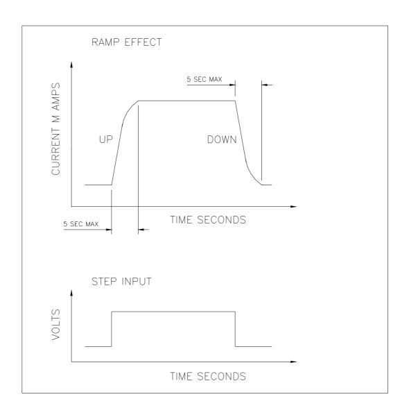
As can be seen for a given step input to the amplifier the output of the amplifier can be adjusted to give a gradual step response.
