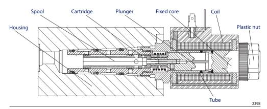
**Coil** is a winding of enamelled copper wire, able to withstand high temperatures and then encapsulated in melted plastic or resin. There could be two wires that exit this plastic covering so that they can be connected externally.
