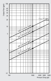
Valve Flow Diagram D634 Series
