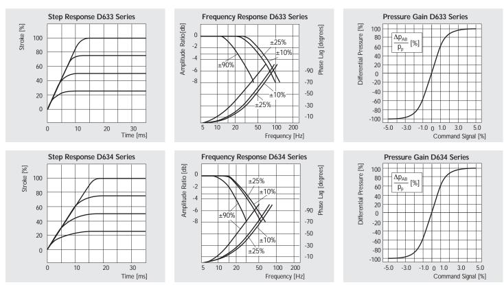
All curves measured at  $p_{S}$  = 2000 psi and a fluid viscosity of v = .05 in<sup>2</sup>
