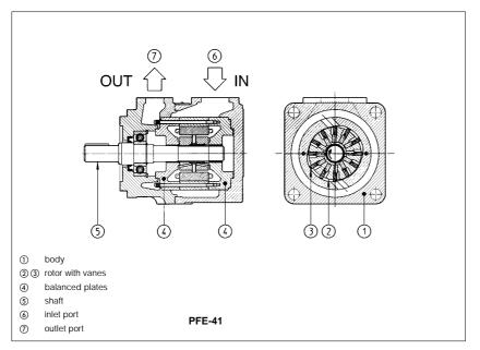
PFE are fixed displacement-twelvevane pumps, ② ③ cartridge design with integral hydraulic balancing (4) for high pressure operation and long service life with low noise level.
