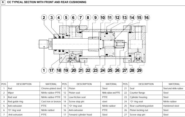
"O" ring seal Nitrile rubber Metering rod Steel 28 Counter flange Steel Forward cushioning piston Hardened steel "O" ring seal Nitrile rubber 29 Rear cylinder head Steel "O" ring seal Nitrile rubber Screw stop plug Steel
