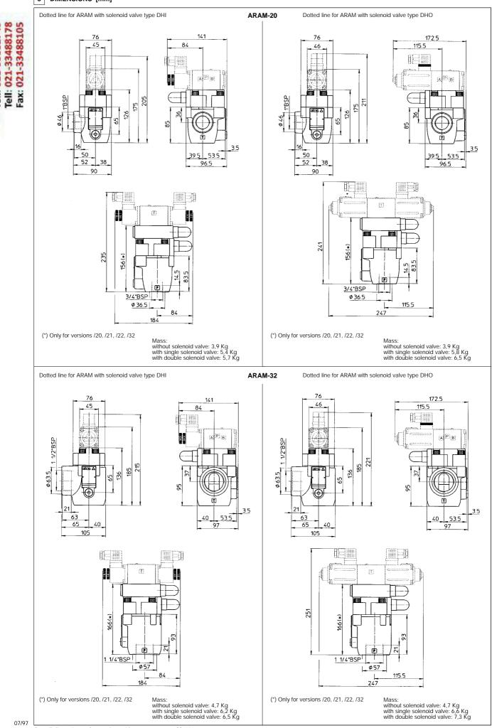
Overall dimensions refer to valves with connectors type SP-666
