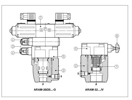
ARAM are double stage pressure relief valve with balanced poppet and BSP threaded ports.
