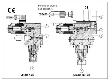
LICZO (compensator), LIMZO (relief) and LIRZO (reducing) are 2-way proportional pressure cartridge valves. They are composed by a 2-way cartridge ① housed in a recess of standard ISO/DIN dimensions. and by a closing cover with a piloting proportional pressure relief valve type RZMO (3), see tab. F007.
