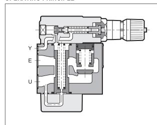
The Z\*-P type valves are used when a branch with a lower pressure than the main one is desired in the hydraulic circuits.
