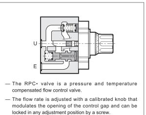
The flow rate adjustment range is carried out with six turns of the knob, with indication of the number of turns made. A one-turn adjustment on the knob, RPC\*/M, is available upon request.
